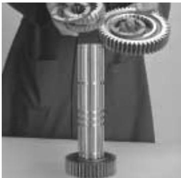
6. Remove the offset washer and sliding clutch, and then remove the offset washer and 3rd gear.
