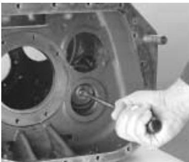
4. From the case rear, insert the idler shaft through the main case bearing bore and into the reverse idler gear bearing.
