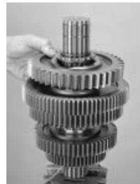
26. At this time remove the air line and insert the mainshaft key. Be careful not to move the gears while doing this procedure, the tolerance washers are unlocked and can rotate which would cause the gears to drop.
