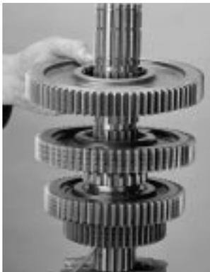
16. With clutching teeth up, install the next gear on shaft against the previously positioned gear.
