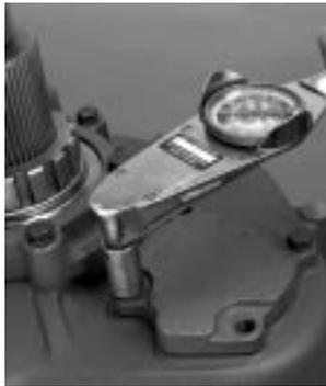
14. Apply Eaton® Fuller® thread sealant #71205 or equivalent to the auxiliary countershaft rear bearing cover capscrews and auxiliary countershaft rear bearing cover.
