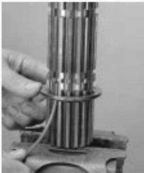
3. With the washer flat side up, position a gear tolerance washer (white) in the mainshaft 1st or bottom groove. Rotate the washer until the washer splines and mainshaft splines align.
