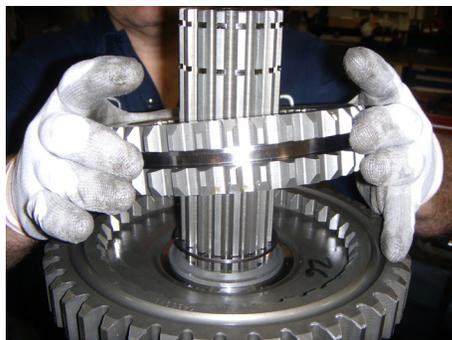
18. Install the snap ring in the mainshaft groove.
