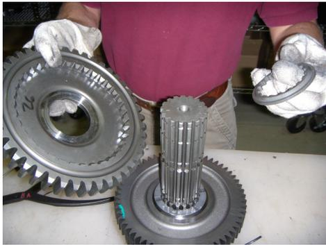
4. Remove the offset washer and 1st gear.
