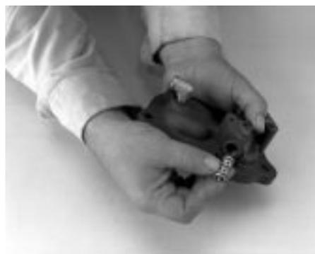
5. Remove the 15/16" nut on the range yoke bar.
