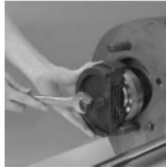
8. Swing the front of the countershaft to the center of the case, and lift out the countershaft assembly.
