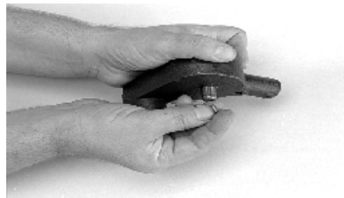
4. From the drive shaft keyway, remove the key.
