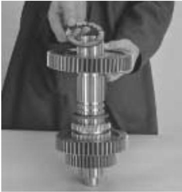
6. Remove the offset washer and 1st gear.
