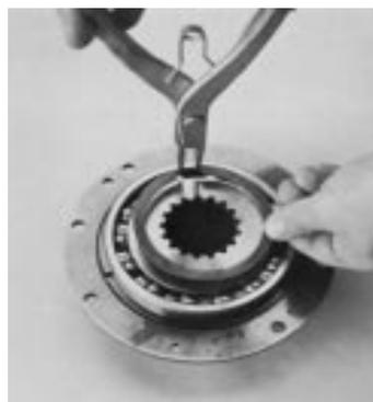
4. Install the outer retainer ring, grooved side down (inset), with a flanged driver.
