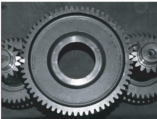
4. Use a round file or bar to properly align from the marked teeth on the Auxiliary Countershaft to the Auxiliary Splitter gear. When the bar is lined up with the root, between the correct teeth, you will notice it's parallel with the Auxiliary Countershaft. Mark both the teeth with a highly visible paint.
