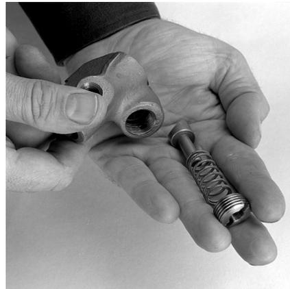
10. Inspect the yoke or block parts, replace the worn parts.
