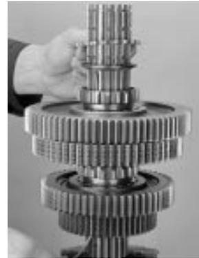
25. Install reverse gear on the mainshaft. Engage the gear clutching teeth with spacer external splines and sliding clutch. Move the reverse gear down against the 1st speed gear.
