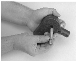
5. If removed, replace the drive shaft snap ring on the pump drive shaft.
