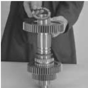
5. Remove the flat washer and 2nd gear.
