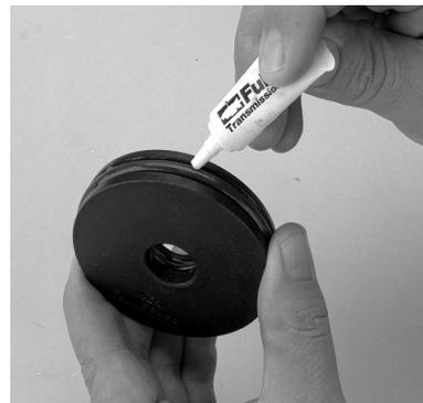
3. Install O-rings onto range and reduction pistons.
