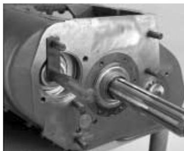
2. Insert the mainshaft hook tool or rope around the mainshaft.
