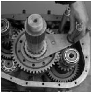
13. Install deep reduction yoke into slot on deep reduction sliding clutch. Make sure positioning is correct.
