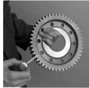
16. Install reduction gear over auxiliary mainshaft. Line up marked teeth.
