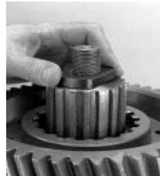
10. If reusing nut, apply a thread locking compound to the threads. New nuts should have a pre-applied locking compound. Torque the nut to 180-210 Lbf-ft.
