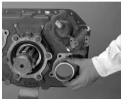
8. If necessary, secure the countershaft assemblies in a vise and remove both the front and rear bearings with a bearing separator and jaw pullers.
