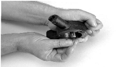
8. From the integral oil pump housing, remove the drive shaft.
