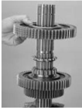
15. With clutching teeth down, position the next gear on the mainshaft engaging with spacer external splines.
