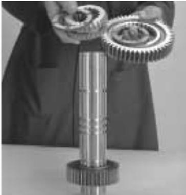
8. Remove the offset washer and sliding clutch.
