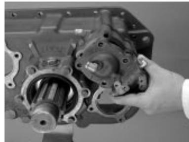
4. If necessary, remove the insert valve retaining nut from the cylinder cover. Remove the insert valve from the bore.
