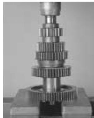
5. Align PTO gear keyway with the countershaft key, bullet-nose of teeth facing up (shaft rear). Align drive gear keyway with the countershaft key, long hub against PTO gear, and press both gears on the countershaft.
