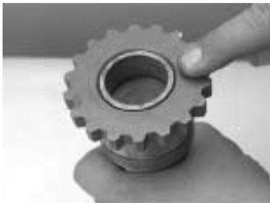
10. Inspect the bushing in the input shaft pocket, replace if damaged.
