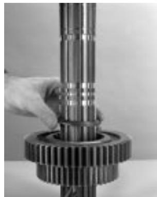
9. Push the air line up to lock the washers on the mainshaft.
