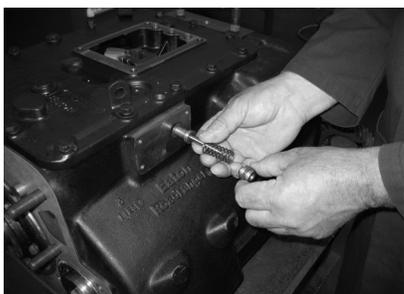
6. Install interlock parts (pin, spring and sleeve).
