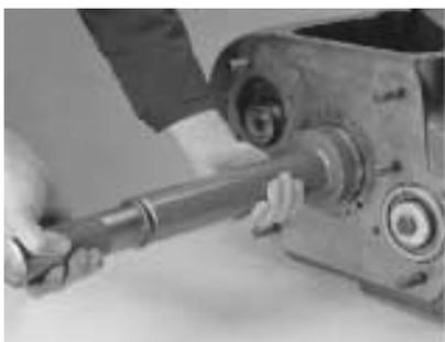
5. Install the input shaft bearing over the input shaft. Use a flanged-end bearing driver which contacts both the bearing inner race and outer race. Drive the bearing until it contacts the front case.
