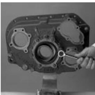
26. Apply Eaton/Fuller Sealant #71205 or equivalent to the retaining capscrews.
