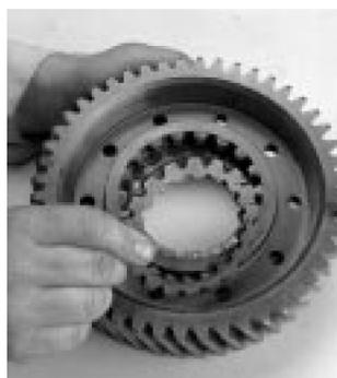
4. Install splined washer in low range gear
