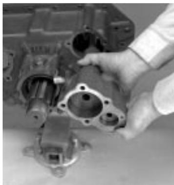
7. Remove the cylinder housing and gasket.
