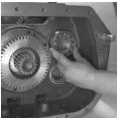
12. From the rear, remove the countershaft support tool.
