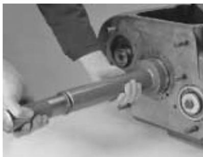
11. Install the input shaft retaining snap ring.
