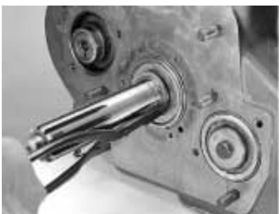
6. Install the input shaft retaining snap ring.
