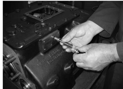
7. Install slave valve. Apply Loctite 242 to capscrew threads and torque to 8-12 lb-ft (10-85-16-30 N•m).
