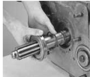
7. Remove the drive gear internal snap ring.
