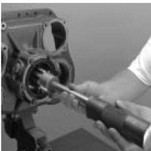
9. Use a soft bar and maul to completely drive the output shaft forward and through the rear bearing assembly.
