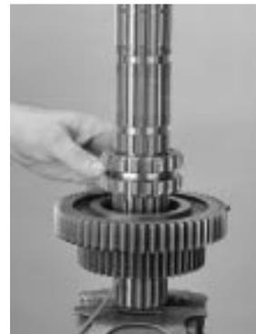
12. With the washer flat side up, position tolerance washer (white) in the next available groove. Rotate the washer until the washer splines and mainshaft splines align.
