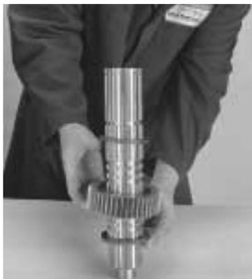
7. Remove the flat washer, remove the 4th or overdrive gear, and remove the offset washer.
