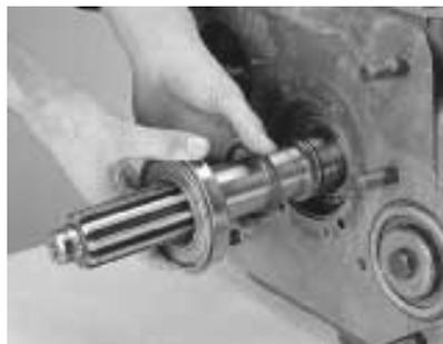
8. Install the input shaft bearing over the input shaft. Use a flanged-end bearing driver which contacts both the bearing inner race and outer race. Drive the bearing until it contacts the front case.
