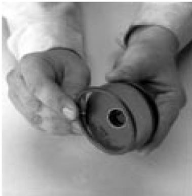
9. If necessary, remove the O-rings from the range cylinder bore and the reduction cylinder bore.
