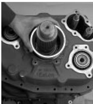
20. Install inner bearing spacer.
