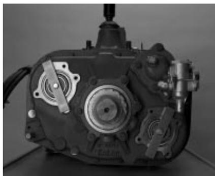
3. Install countershaft retaining strap.
