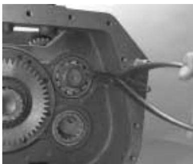
14. In the countershaft rear groove, install the rear snap ring.
