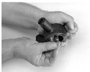
7. Install the two (2) keys on the drive shaft.
