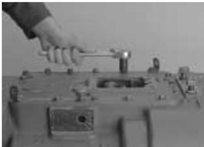
4. From the shift bar housing rim, remove the retaining cap-screws.
