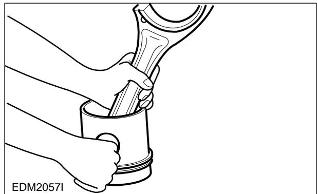
On the piston head surface, the longer side of conn. rod big end is in opposite direction from the valve seating surface as well as in the same direction with the narrow margin of combustion chamber.
