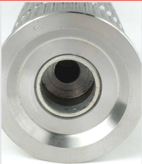
J. Inspect the output shaft bushing for damage.
