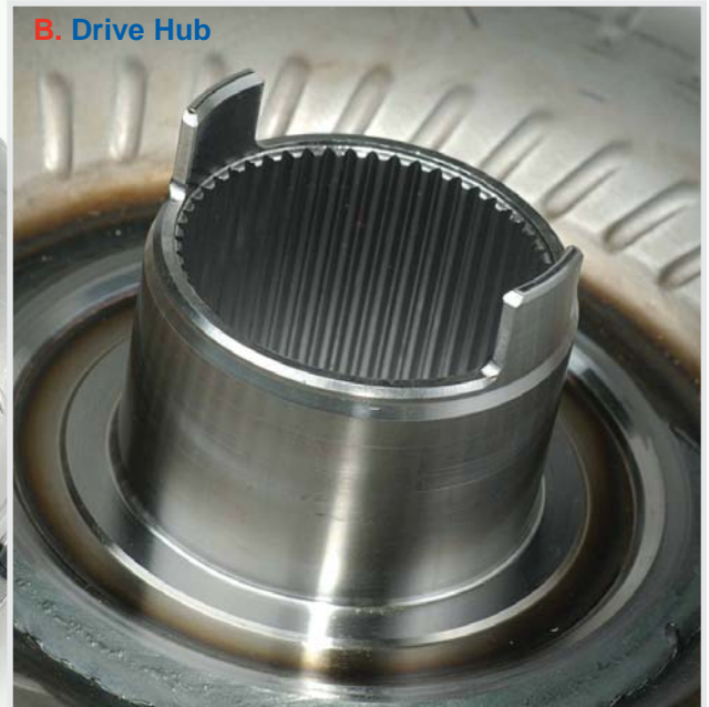
Inspect the pump hub tangs for cracks, impact damage and broken tangs.
