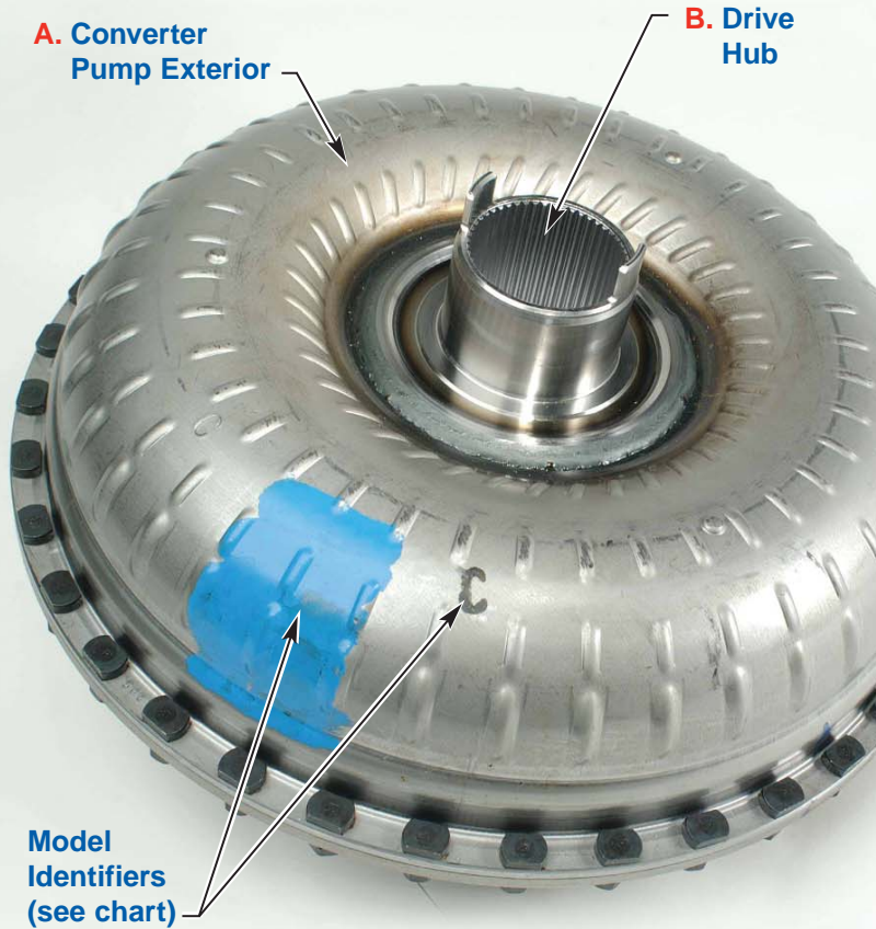
Inspect the pump hub tangs for cracks, impact damage and broken tangs.
